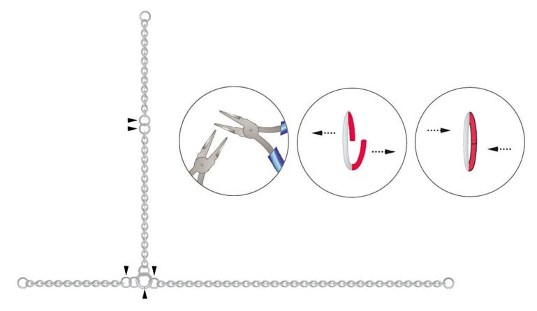
STEP 4: Cut a 10 cm piece of 1 mm gauge wire and wind it around a pen or pencil of approximately 10 mm thickness. Cut through this spiral to get a 12 mm jump rings as shown in the illustrations.
